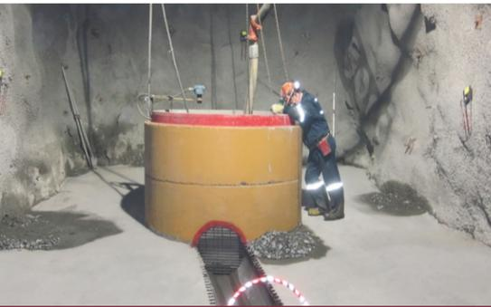
Bomba sumergible de GPM-Eliminator & Sumidero "Wilson"
